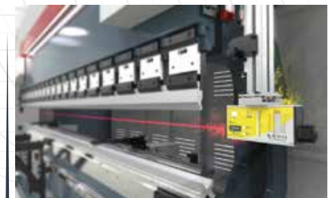
CE Laser Safety System
