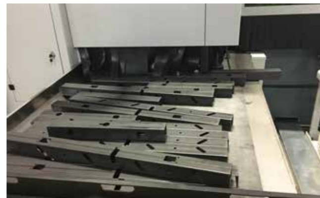
Tubes up to 236,2 of length are removed by automatic unloading system with conveyor.
