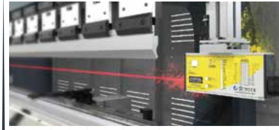
CE Laser Safety System
